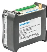
The Gunnebo Bridge is the gateway which securely routes communication between a group of Gunnebo products and the cloud.
